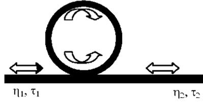
Fig. 1. A SRL with its directionally coupled straight waveguide. Feedback occurs at the end-facets of the waveguide.
