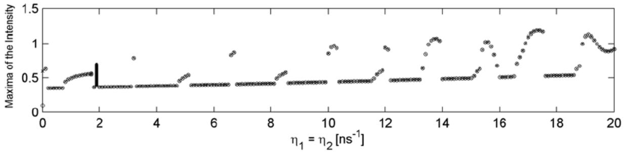
Fig. 2. Bifurcation diagram for the intensity. The maxima of the clock-wise mode (x) and of the counterclockwise mode (o) are recorded.
