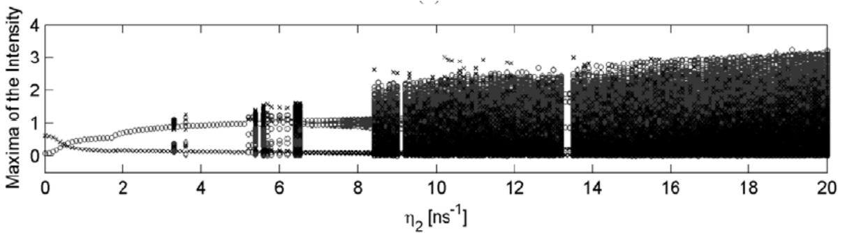
Fig. 3. Bifurcation diagram for the intensity. The feedback strength  $\eta_1=0.5\text{ns}^{-1}$  is fixed, ( $\Theta_1=\Theta_2=\pi$ ). The maxima of the clock-wise mode (x) and of the counter-clockwise mode (o) are recorded.
