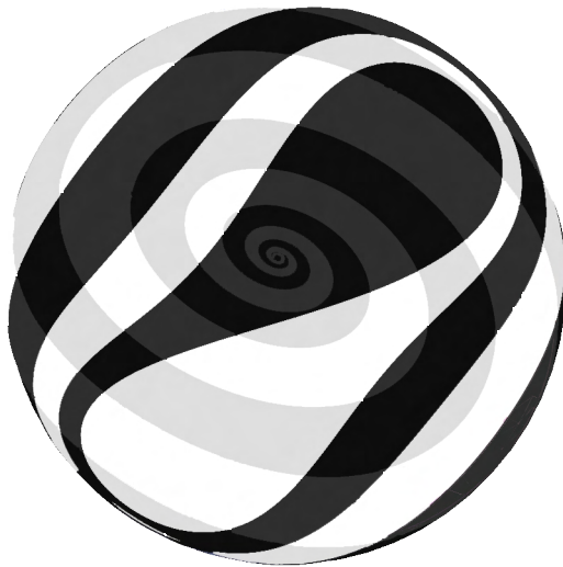
The basins of attraction of both counter-propagating modes of a semiconductor ring laser plotted on a sphere (Courtesy of Vincent Ginis).
