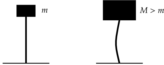
Figure A.3: Beam buckling. At a certain mass M , the vertical position becomes unstable and the beam may buckle (figure based on [1])
