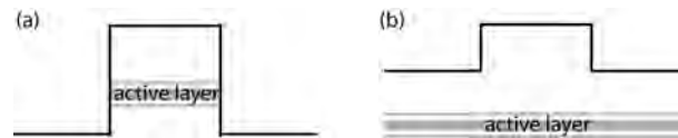
Figure 1.6: Schematic representation of (a) a rib waveguide and (b) a ridge waveguide.
