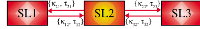
FIG. 1. (Color online) Open-end scheme of three mutually coupled semiconductor lasers interacting bidirectionally with a time delay.
