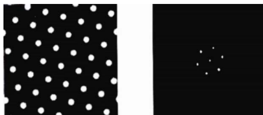
Figure 1.6: Hexagonal pattern produced by the intensity of two counterpropagating beams that have crossed a rubidium cell [146]
