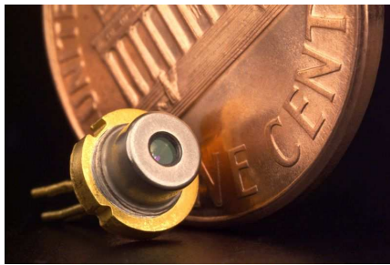
Figure 1.3. Typical semiconductor laser with its package capsule.
