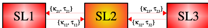
Figure 8.1. Open-end scheme of three mutually-coupled semiconductor lasers interacting with a time delay.
