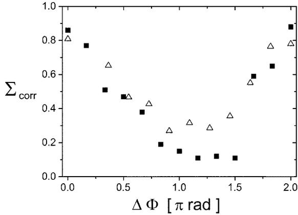
Fig. 3. Experimental cross-correlation coefficients of the intensity time series of transmitter and receiver versus the relative optical feedback phase  $\Delta\Phi$  under LFF operation ( $I_{t,r} = 1.01 I_{th,so1}$ , solid squares), and CC operation ( $I_{t,r} = 1.15 I_{th,so1}$ , open triangles), respectively.
