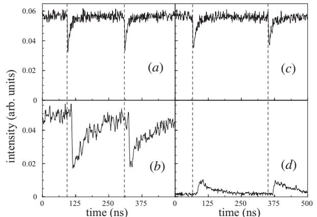
**Figure 2.** Modal structure of a dropout. Total intensity evolution (a), (c) compared with that of the main mode of the laser with feedback (b) and of the original main mode of the solitary laser (d). Traces (a), (b) and (c), (d) have been acquired simultaneously (but note the intrinsic delay of the mode-selecting path of the set-up—see text). Vertical dashed lines are a guide to the eye.
