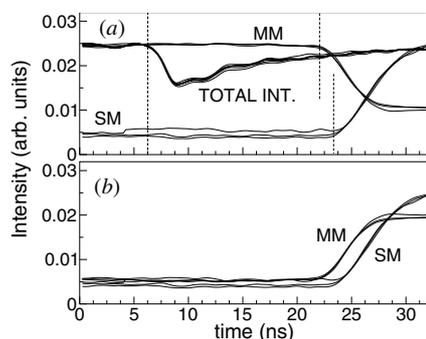
**Figure 3.** Averaged time traces of a dropout in the total intensity, MM of the laser with feedback and MM of the solitary laser. In plot (b), the traces of the MM have been inverted.
