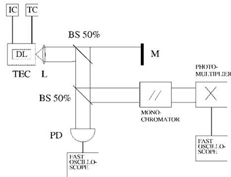
**Figure 1.** Experimental set-up: DL, laser diode; BS, beamsplitter; M, external mirror; TEC, laser diode mount; PD, photodiode; IC, intensity controller; TC, temperature controller.
