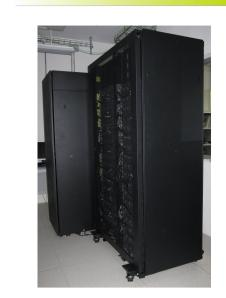
Nuredduna, the main tool for High Throughput Computing at IFISC, is composed of two parts: a cluster designed and build at IFISC which with 200 computational cores, and a grid cluster with the Grid-CSIC initiative to promote e-science. The grid cluster includes an IBM iDataplex with 512 computational cores and 96TB of raw storage.
